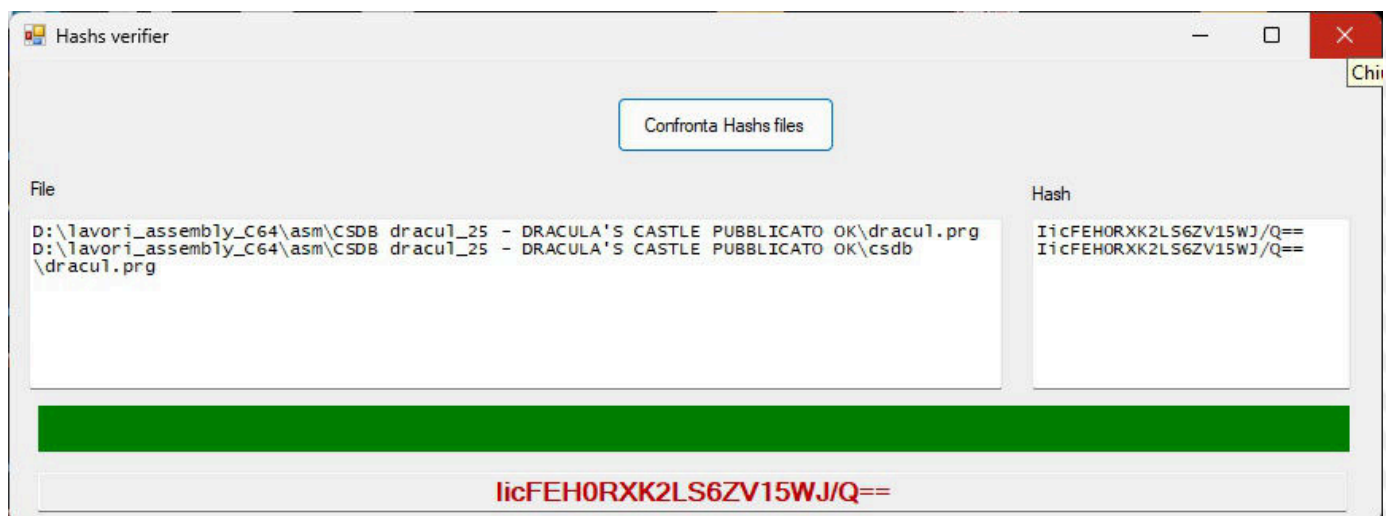
Fig. B - Comparison of the MD5 HASH of the game I published on CSDB "Dracula's Castle" in 2017 with the one I recently recompiled. The comparison result is positive, so the two .prg files are absolutely identical, down to the last byte
