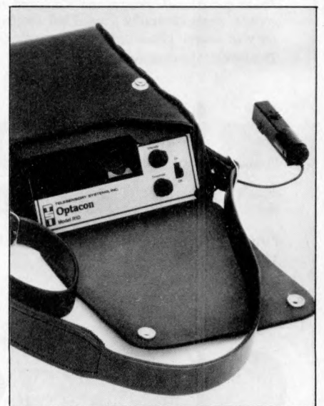
The TSI Optacon, with its miniature camera to the right. The tactile 'reading' pad is visible inside the slot.
