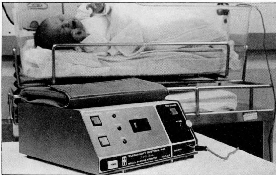
The neonatal screening audiometer is designed to detect hearing deficiencies in newly-born babies.
