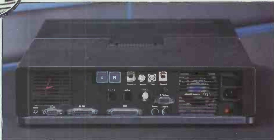
The rear of the Dynamac has been utilised to the limit. Most ports have been inherited from the Mac Plus, with additional slots for an internal modem and networking facilities.
