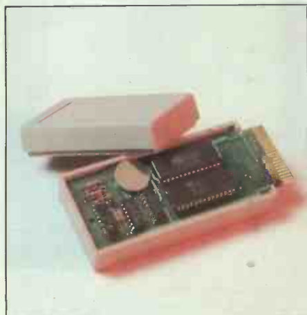
The hardware of McEmulator is nothing more than a standard ST ROM cartridge without any ROMs. McEmulator Plus, shown here, also has a real-time clock
