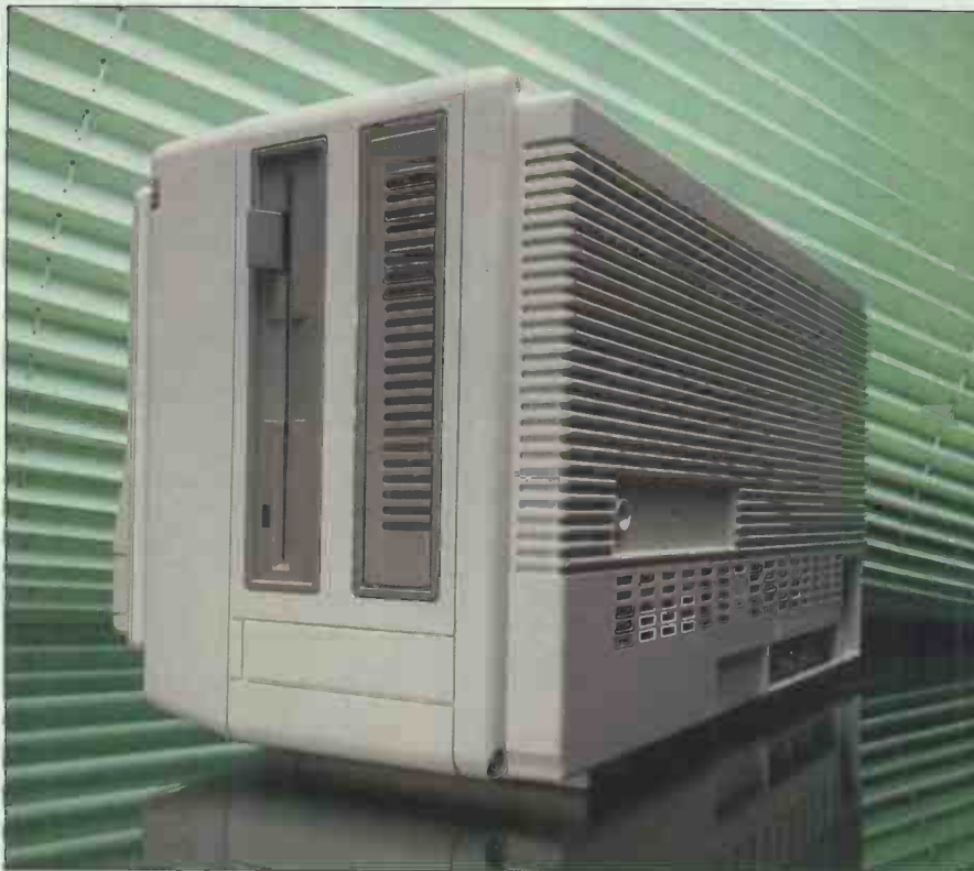
One of the major reasons for the Compaq's 'larger-than-lapheld' design is the inclusion of a standard 5¼in disk drive
