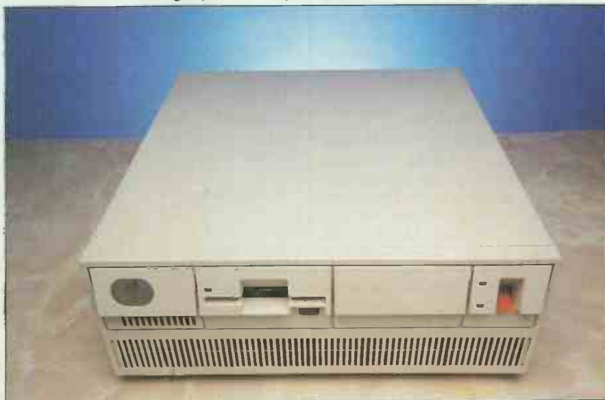
The new machines lack the bulk of previous PCs and the 3½in disk drive may now be here to stay. The mains switch — a clumsy affair — has migrated to the front while the keyboard lock is now on the back
