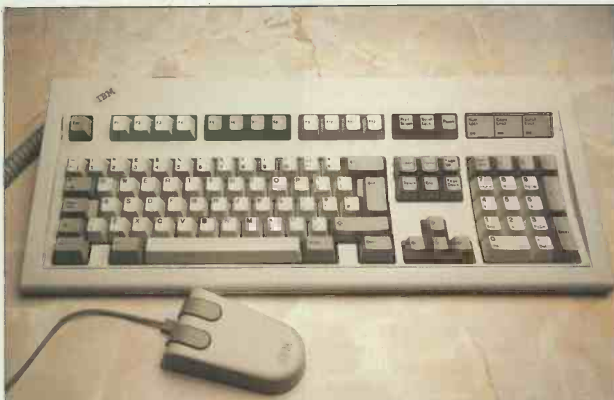
Reinforcing the AT/E as the standard PC keyboard, the 102-key unit includes a separate cursor and numeric pad — and twelve function keys seems to be the new gospel. The stylish mouse is a standard item
