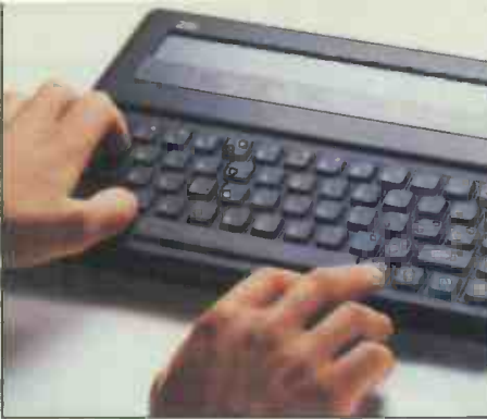
Full QWERTY keyboard offers 'silent', moving short-travel keys. Foldaway foot raises the Z88 12½" for comfortable viewing and typing.
