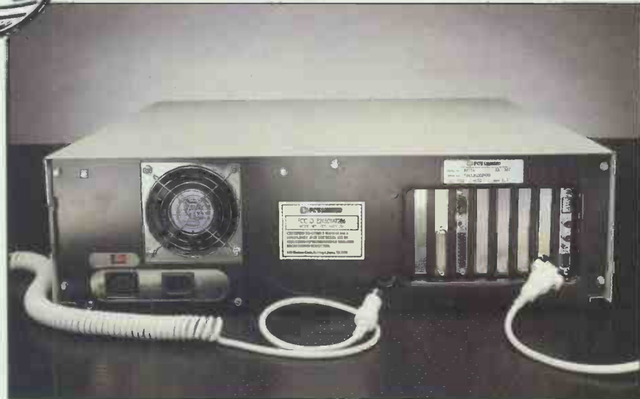
The system comes with an EGA card, a parallel printer port and two serial ports as standard. The power supply is rated at 200 watts, so you can save a mains socket by connecting the monitor directly to the computer
