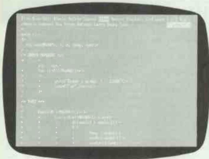
Zorland C offers an integrated environment similar to Mix C and Turbo C, but uses 1-2-3 style 'across the screen' menus without windows
