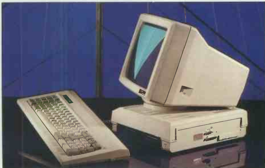
Twin 3½in floppy drives, mouse and parallel ports are the minimal external access points available. The expansion port allows for the addition of a serial port and/or modem
