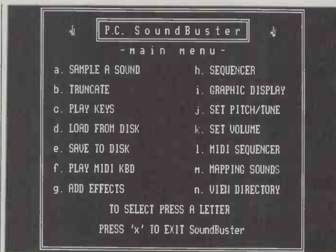
The opening menu of the PC SoundBuster system lists operations for sampling a sound and for editing a sequence
