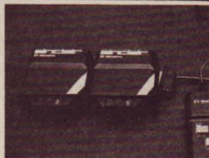
Top, shows use of PAPER command; below two 100K Microdrives, out later.
