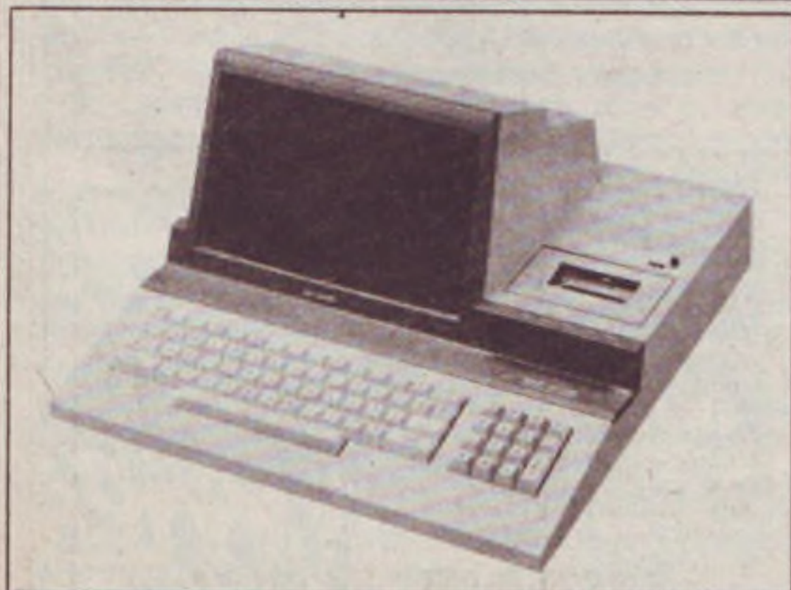
The new Sharp personal computer with 48K RAM. The MZ80A has a standard keyboard, green CRT display and a cassette deck in one self-contained unit. The basic price is £549. More details are available from Sharp on 061-205 2333.
