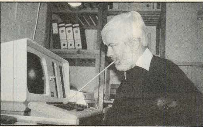
Two word-processing systems: WordStar can be accessed using a mouthstick, and MacApple, a pedal-operated system.
