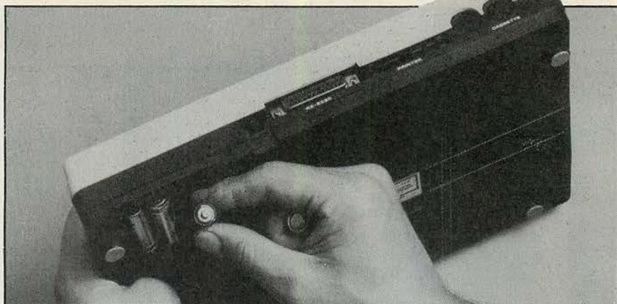
Four AA batteries power the Tandy 100, with rechargeable back-up to maintain RAM.
