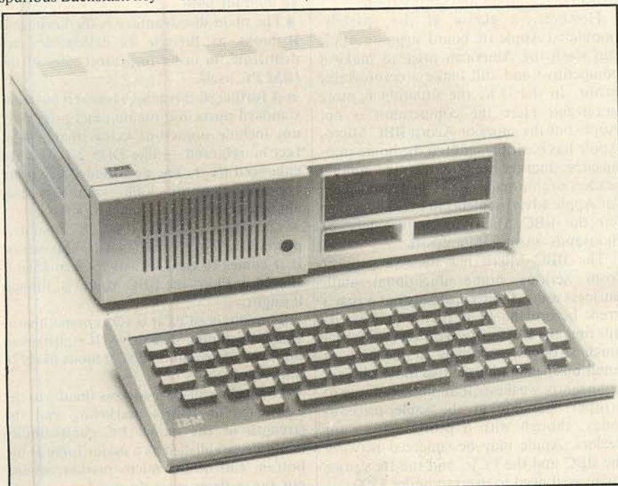
The PCjr is a downgraded model, and there are 21 fewer keys than on the PC.
