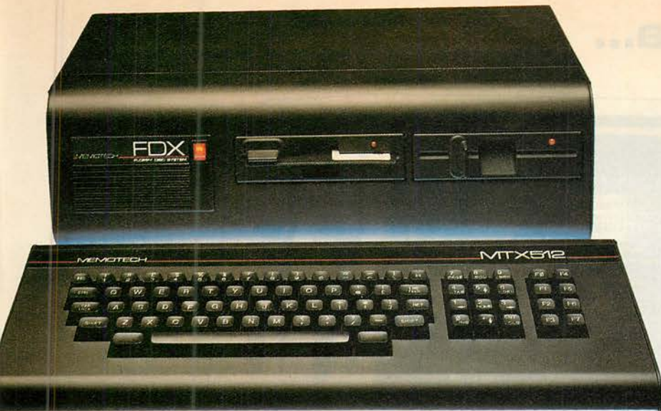
MTX512 plus twin 5 1/4" disc FDX. A CP/M based business system - £1245 inc VAT.
