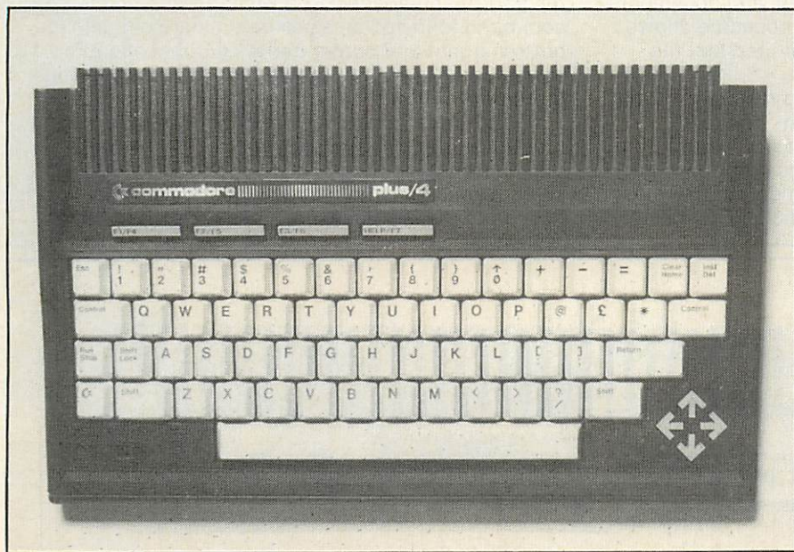
The Plus-4's switch-like function keys are easy to use, as are the neat compass-point cursor-control keys.
