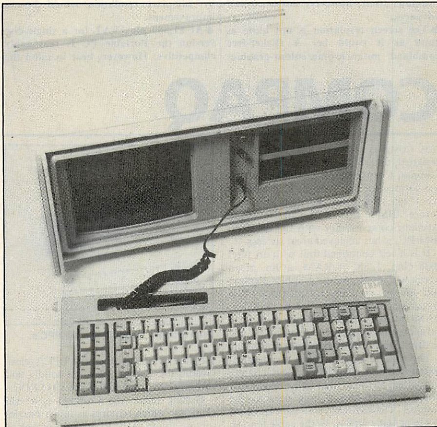
The PPC keyboard has the same layout as the desk-top version but is smaller.
