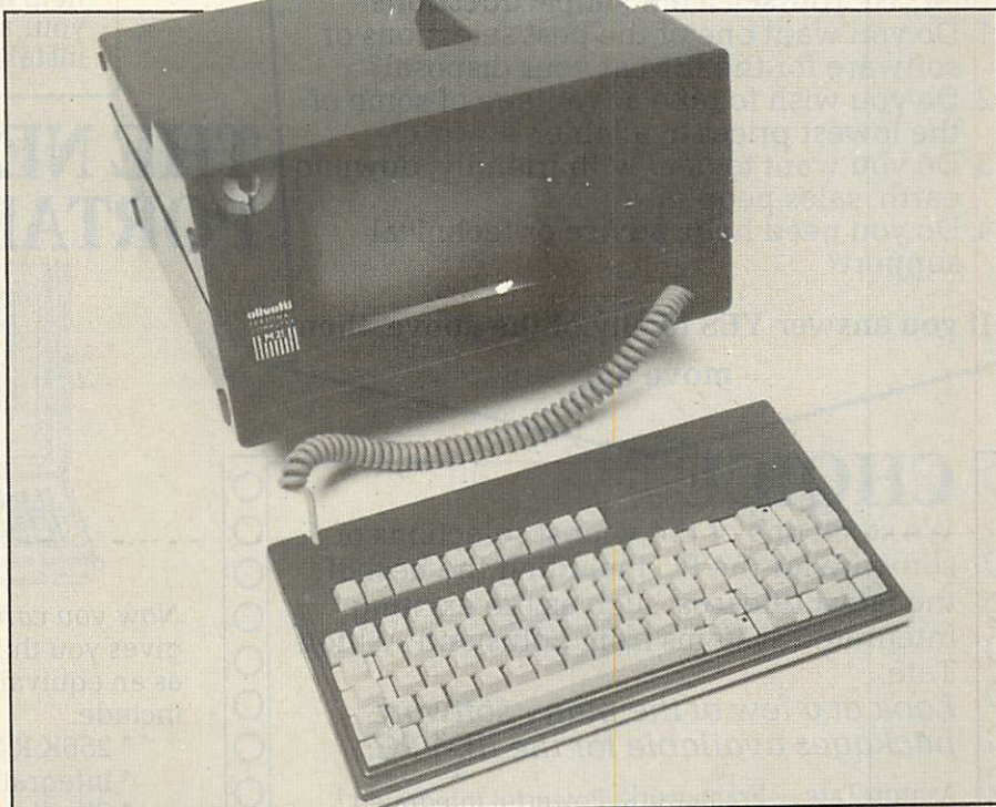
The oddly-shaped M-21 has its function keys across the top of the keyboard.
