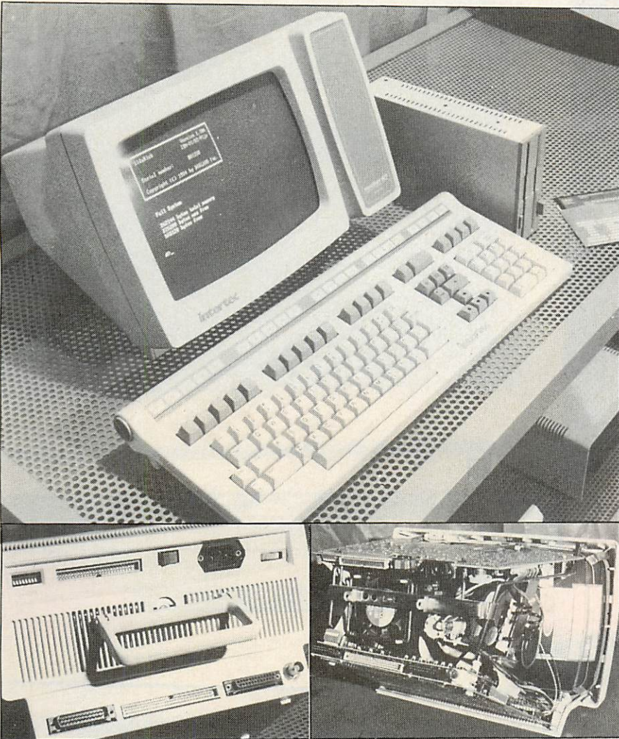
Top: Headstart has the same character definition set as the IBM PC's green screen. Above left: the expansion ports lie at the back of the screen/system box. Above right: the electronics are packed tight inside the VDU casing, leaving no room for expansion cards.
