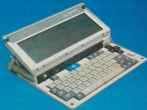
A large, legible screen was one of the requirements revealed by a CCTA study. Accordingly the Liberator has a clear, 16-line by 80-column LCD display.
