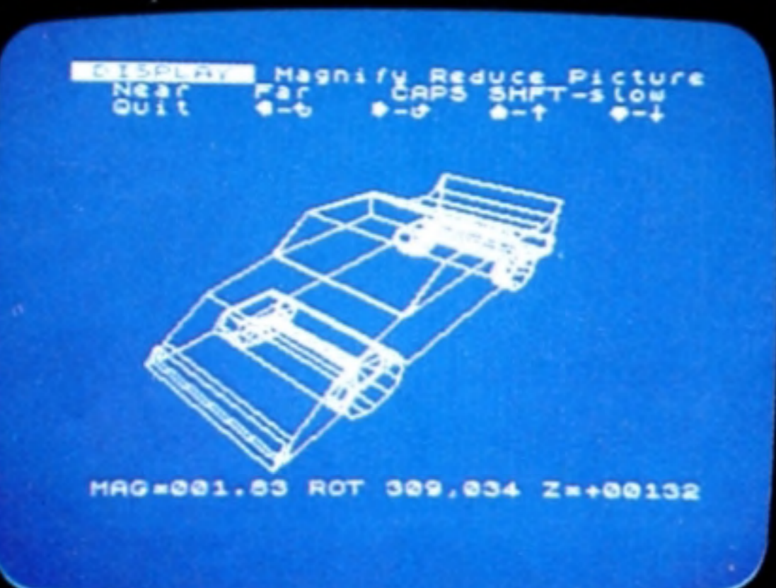
Problem. Modelling in 3-D on a small micro - performing some 7.5 million calculations for one hidden line drawing.
