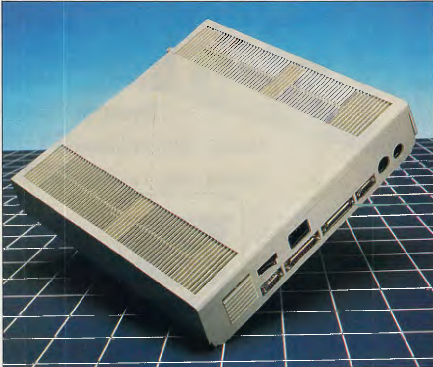
The array of back-panel connectors includes a complex DIN socket for an external floppy drive; this also appears on the ST range
