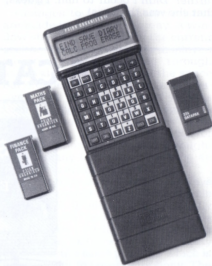
The Organiser II with some of the packs which slot into locations on the back. Overall length is actually to the bottom of the keyboard, the remainder being a sliding protective cover which can be removed entirely.
