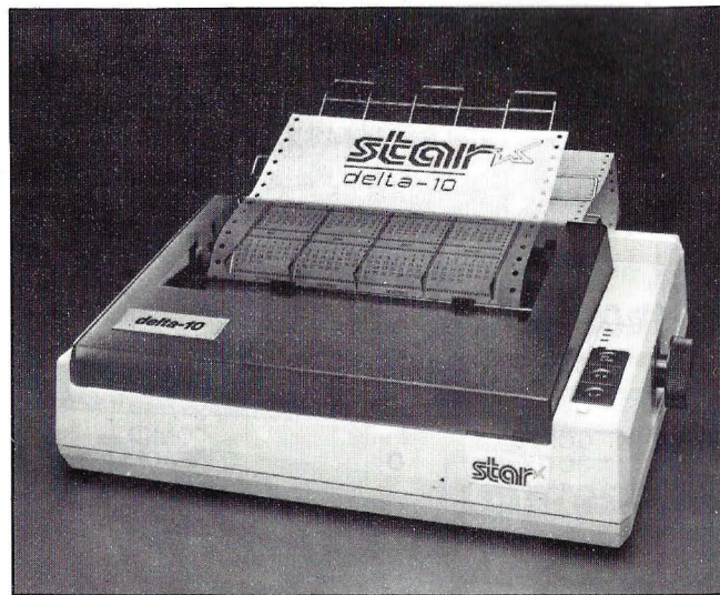
Delta 10 : 80 columnas, 160 cps. Delta 15 : 132 columnas, 160 cps.
