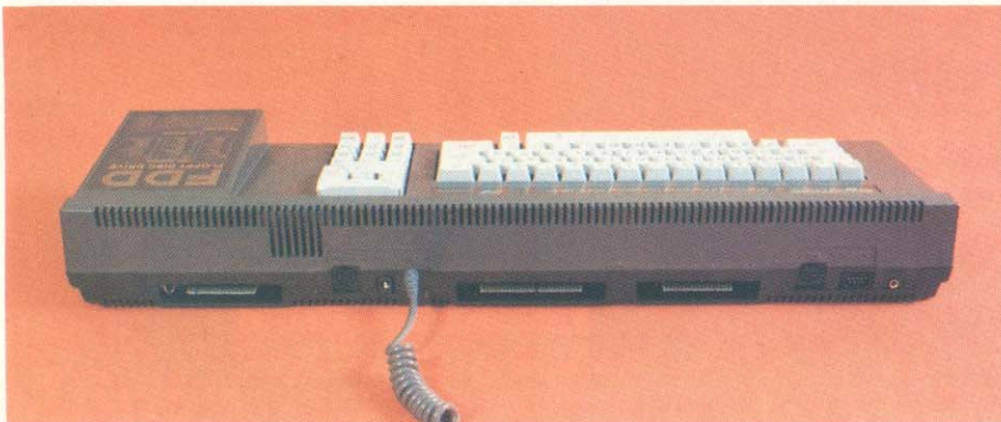
Anschlüsse (v.l.n.r.): Floppy/Monitor/5V/12V/Expansion Port/Drucker/DIN-Anschluß für Recorder/Joystick/Stereo
